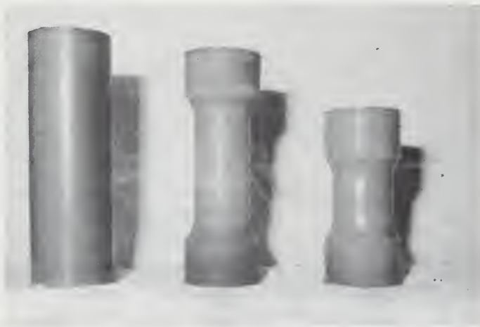
FIGURE 2. BIAXIAL SPECIMEN MACHINING PROCESS. SHOWN LEFT TO RIGHT, HOLLOW CYLINDRICAL CASTING, MACHINED BIAXIAL TENSILE SPECIMEN, AND MACHINED BIAXIAL COMPRESSIVE SPECIMEN.
